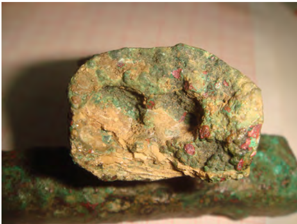
Fig.11: Detail of broken casting funnel IVA.64, showing the bubbles produced by gases during casting
