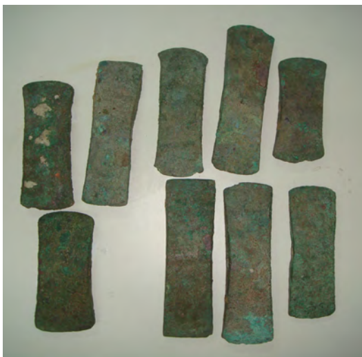
Fig. 3: The axes from the Merchant Hoard. In all examples one blade is hammered, the second is left in as-cast condition
