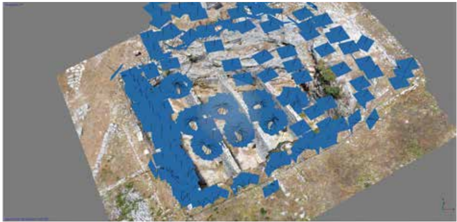
Figure 6.9a: Finnish Institute Three-Dimensional Development Programme, 2016. Hellenistic reservoir at Pleuron. Combining land-based and aerial digital photography to produce three-dimensional models using photogrammetry. Model with locations of the UAV and hand-held camera photographs indicated by blue rectangles (image by Jari Pakkanen).
