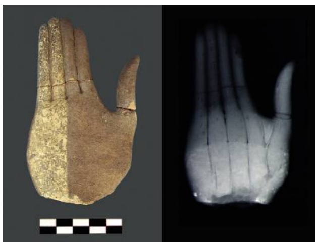
Fig. 8 X-radiograph of a representative palm of group A showing the difference in the grain size of the clay used for the arm-forearm-palm and the finger coils. Faxitron 43855A, 56 cm focus-to-film distance, 40 kV, 7 min, 3 mA.
