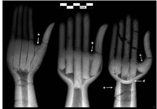
Fig. 6 X-radiograph of hands of Groups A (left), B (middle) and C (right). Faxitron 43855A, 56 cm focus-to-film distance, 100 kV, 1 min, 3 mA.
