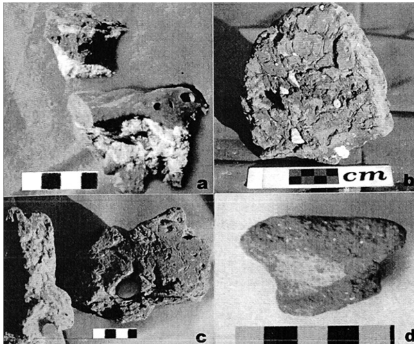
Fig. 11. Sideri (Kythnos): a) Copper slag, b) Fragment of metallurgical furnace wall, c) Furnace fragments with perforations, d) Conical clay nozzle (internal side) (BASSIAKOS-PHILANIOTOU 2007).
