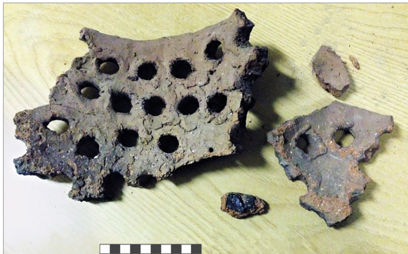
Fig. 16. Fragments of the internal surface of the reconstructed perforated furnace wall after the smelting experiment. The upper part of the furnace with the rim and slag traces, perforated fragments and fragment with slag (Courtesy Dr Bassiakos, Laboratory of Archaeometry 'Demokritos' NCSR).
