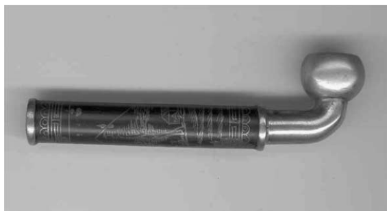
Fig. 1. Opium pipe from Kun Ming, Yun Nan, China 19th century A.D. The head is of Ag, the tube is of brass covered by a wu tong sheet of Cu, with 0.6% Au, 1.8% Ag, 1.9% Zn and 0.4% Fe, black patinated by sweaty hands.
