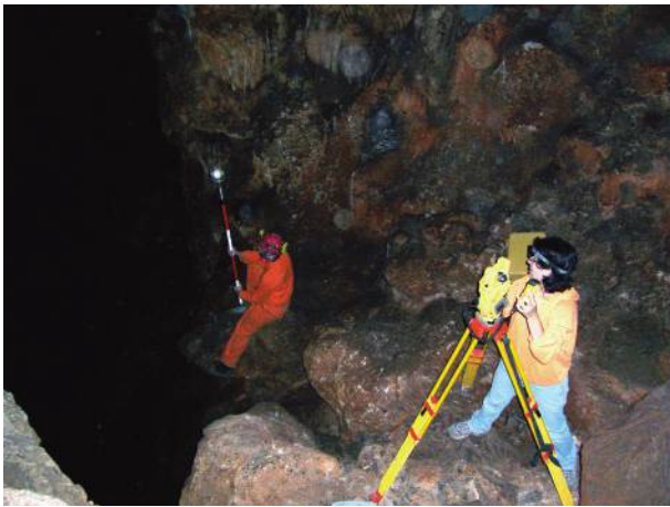
Figure 7 Using the TopCon GTS-303D EDM total station and prism on uneven ground in Skoteino Cave. Photograph by J. Frey.
